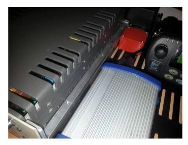
The Isolation transformers are in a small 2" square dicast box (red in the picture to the left).
