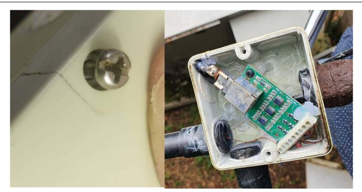
With the cover now fully removed I quickly saw the problem. The antenna box was full to the brim with water and the surface mount PCB was almost fully immersed apart from one small part. This part contained the Amplifier IC and was still working, the rest was under water and it was clear this was the problem. The small desiccator that was added to help keep any damp out was also under water; clearly it had not done its job!
