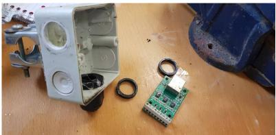
Mat also contacted the company that supplied us the water proof box, who were kind enough to replace it free of charge. So the new Mk2 Antenna box was constructed, which now includes a drain hole, just in case.
