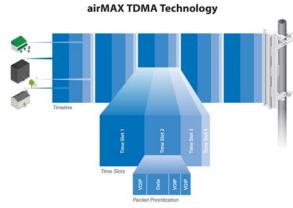
Up to 100 airMAX stations can be connected to an airMAX Sector; four airMAX stations are shown to illustrate the general concept.
