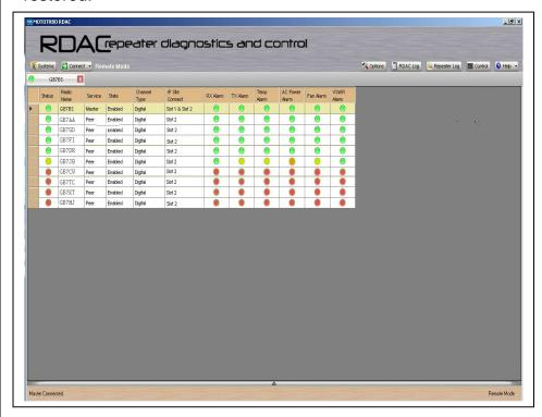
The SWC also has a facility to monitor individual repeaters connected to it and their health. This checks and monitors for any events ranging from a high VSWR to the cooling fans have a problem.
