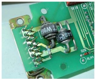
Actual alarm board with the failed diode.
