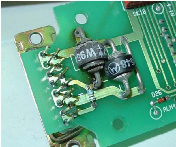
**Actual alarm board with the failed diode.**
