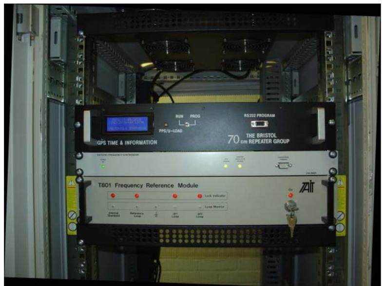
New GPS Clock unit at the top, GPS frequency standards below
